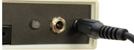
Before connecting the fiber-optic cable into the Power Control Module, make sure that the ends of the cable going into the PCM are not frayed or distorted . If the ends of the cable do not look like they have a straight cut on them you will need to cut them with the cable cutter provided.
