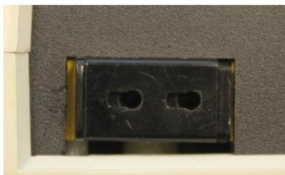
With the ends of the cable cut, open the fiber-Optic cable connector by sliding the left end Of the connector to the left opening up the Holes for the cable.
