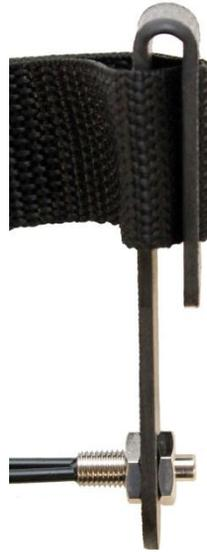
Insert the end of the Fiber-Optic Sensor that you removed the nut from into the plastic holder as show above and replace the nut loosely but so that the Fiber-Optic sensor will not be able to move around. You will still need to adjust the sensor closer to the side of the eye while it is on the end-user.
