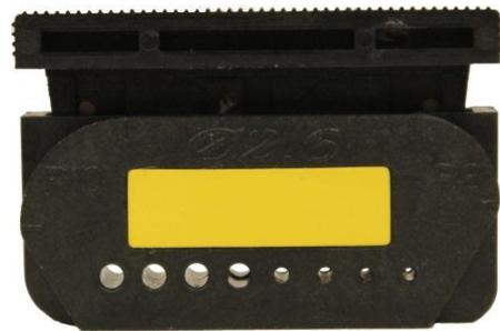
Lift the top of the cutter up so that the blade is Elevated and the cable can be inserted.
