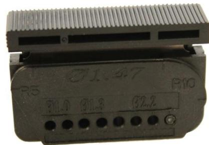
The end of the cable should be seen at the back of the cutter. Push down all the way on Top of the cutter and repeat with the other cable.
