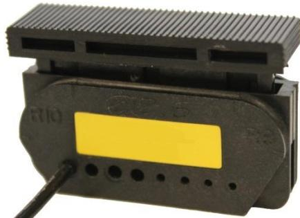
To cut the end of the cable to clean the edge, Insert the end of one of the cables into the hole Of the cutter, the larger hole on the end.
