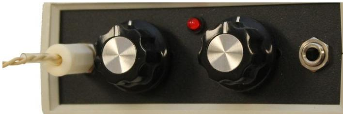
Set the power switch to either ON w/Tone or ON No Tone. With the power switch set to ON w/ Tone you will hear a beep from the Power Control Module each time the sensor is activated. With the power switch set to ON No Tone you will not hear a beep from the Power Control Module
