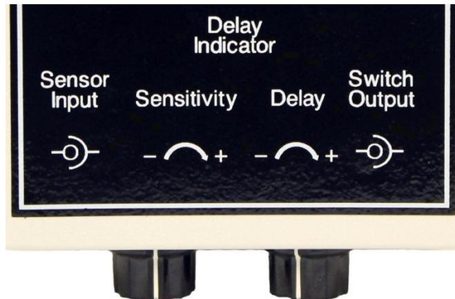
When the sensor is activated the Delay Indicator will light. The LED will stay on for the duration of the delay time. Once activated all activation will be ignored until the LED turns off
