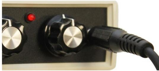
Connect one end of the Piezo Sensor into the jack on the Proximity Control Module labeled SENSOR INPUT.
